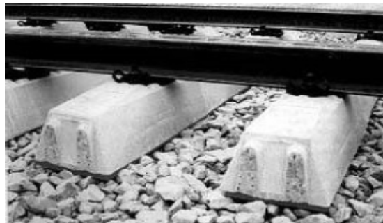
(c) Anti-vibration Roadbed
