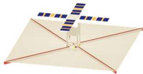
Fig. 3. CNUSAIL-1 Sail Deployment Model
