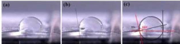
Figure 3. Static contact angle of polyvinylidene fluoride plate; (a) original photo, (b) normal method, (c) Pythagoras rule method.
