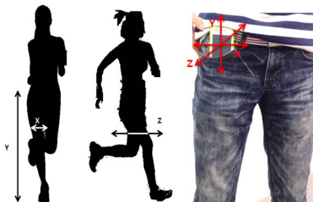
Fig. 8. Direction of the accelerometer
