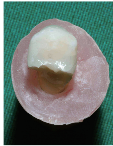
Fig. 3. Mode of unrestorable fracture.
