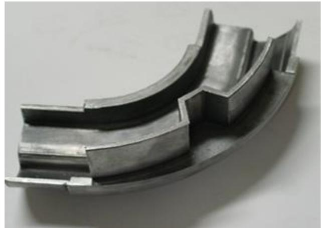
Fig. 7 Appearance of thixoformed A357 roof joint node
