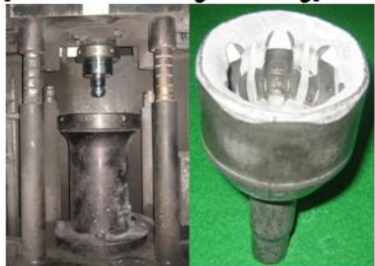
Fig. 9 Multi-stage cold forging experiments for outer race of CV joint
