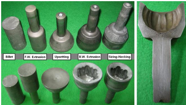
Fig.10 Preforms and prototype of outer race using multi-stage cold forging process
