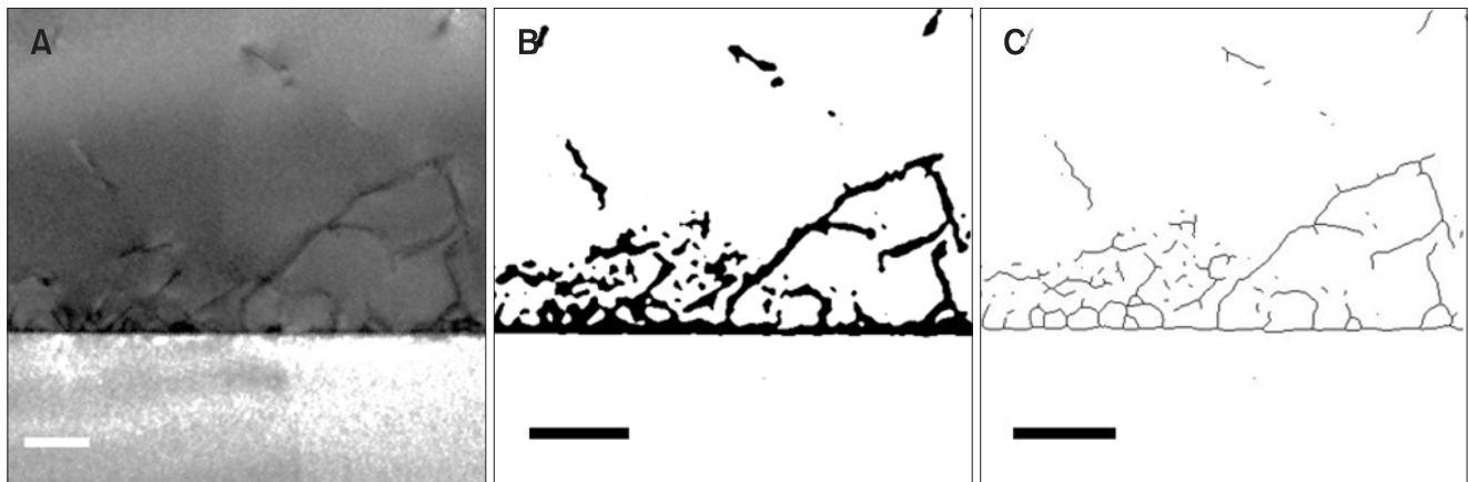
Fig. 2. Image processing steps for dislocation analysis. (A) Dislocations in transmission electron microscopy image of GaAs on Si. (B) Stamp filtered image by Photoshop ver. 8.0 (Adobe Systems Inc.). (C) Skeletonize filtered image by Image J (National Institutes of Health). Scale bars=0.2 \mu\text{m} .
