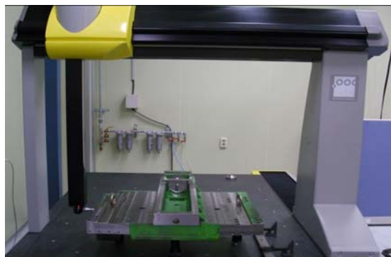
Fig. 7 Photograph of CMM for measuring flatness, parallelism, perpendicularity.
