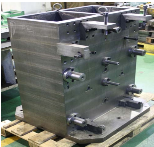
Fig. 6 Photograph of machined Jig & fixture for ultra-precision saddle machining
