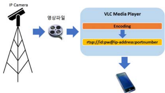
Fig. 10 Flow of IP camera monitoring system
