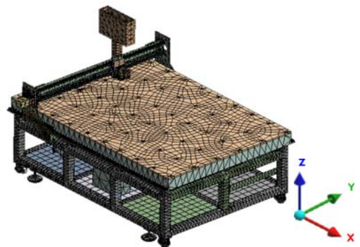
Fig. 8 The simulation model for the analysis of the glass cutting machine
