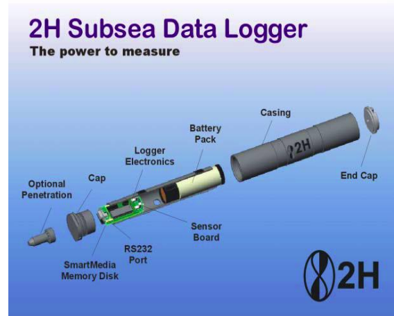
Figure 3. General architecture of a subsea data logger system.
