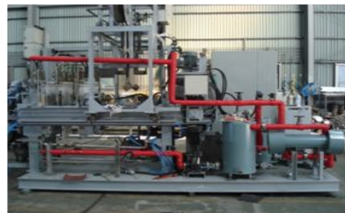
Fig. 3 Schematic diagram and photograph of thermal dewatering: (a) working method of thermal dewatering, (b) photo of thermal dewatering
