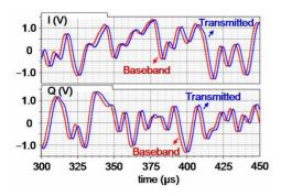
Fig. 11. I/Q components of 8PSK: transmitted vs. baseband.
