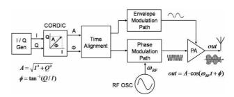
Fig. 1. Block diagram of polar transmitters.
