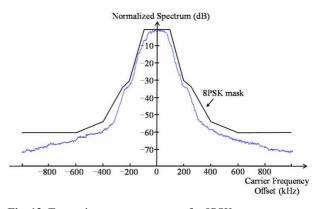
Fig. 13. Transmitter output spectrum for 8PSK.
