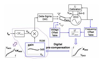
Fig. 5. Proposed digital compensation for VCO tuning curve.
