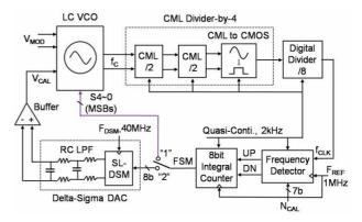
Fig. 6. Proposed dual-mode low-power  $f_C$  calibration loop.
