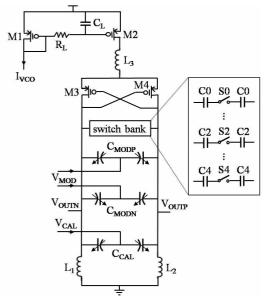
Fig. 4. Proposed three-terminal pseudo-differential VCO.
