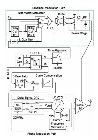
Fig. 2. Proposed polar transmitter.
