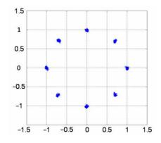
Fig. 12. Transmitter output constellation for 8PSK.
