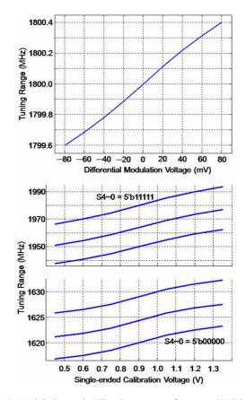
Fig. 7. Modulation and calibration curves of proposed VCO.
