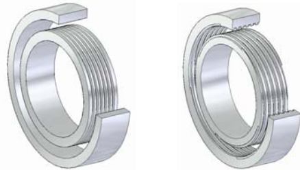
(A) Smooth-Stator/ Parallel-Grooved-Rotor (B) Spiral-Grooved-Stator/ Spiral-Grooved-Rotor
