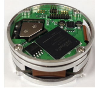
Fig. 2. Shape of the MEMS ISA.
