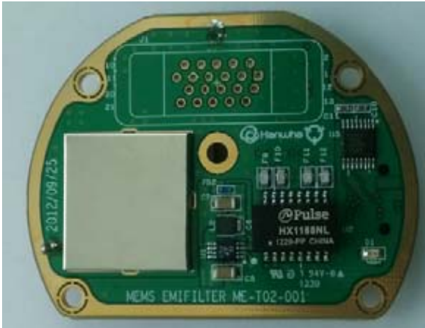
Fig. 6. Shape of the EMI filter board.
