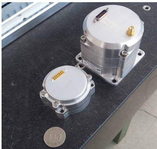
Fig. 10. Shape of the MEMS-IMU/GPS integrated navigation system.
