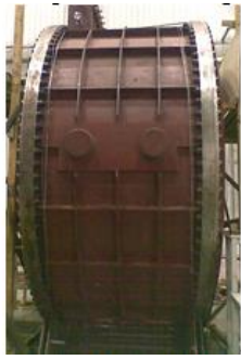
Fig. 5. 2MW direct-driven wind power generator with immersion evaporative cooling system
