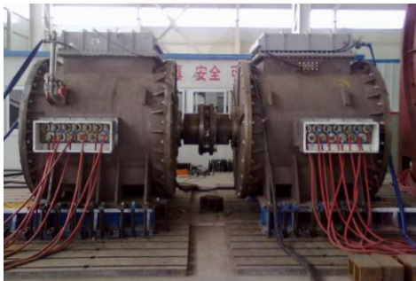
Fig. 6. Two 3.6MW half-direct driven wind power generator with immersion evaporative cooling system in testing
