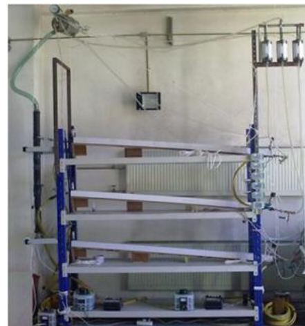
Fig. 9. Experimental facility for two-phase flow instability research in inclined rectangular hollow conductors
