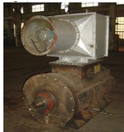
Fig. 4. 1MW brushless doubly-fed wind power generator with immersion evaporative cooling system
