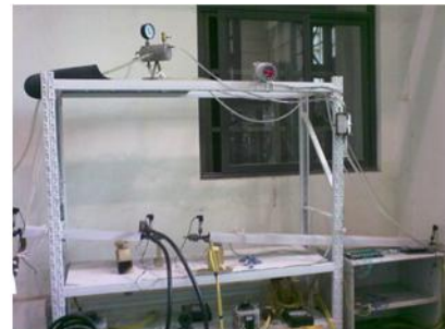
Fig. 8. Experimental facility for two-phase flow frictional pressure drop research in inclined rectangular hollow conductors
