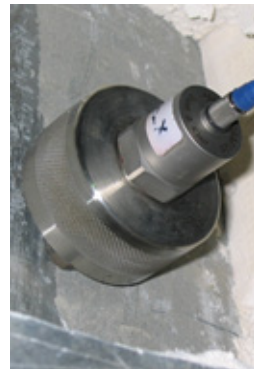
Fig. 2 Attachment of an accelerometer on the pipe using a neodymium magnet having 530 Newton of magnetic force
