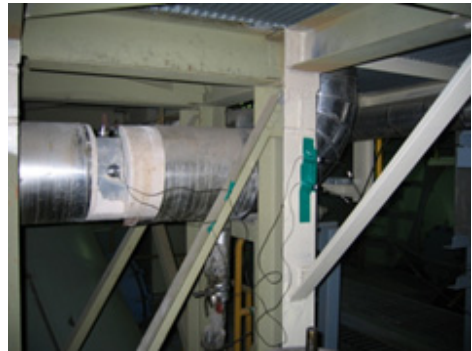
Fig. 1 Two accelerometers attached on the pipe for measuring pipe accelerations in vertical and to-and-fro directions
