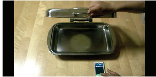
Fig. 9 Photograph of measurement of closing time of lid according to interferences
