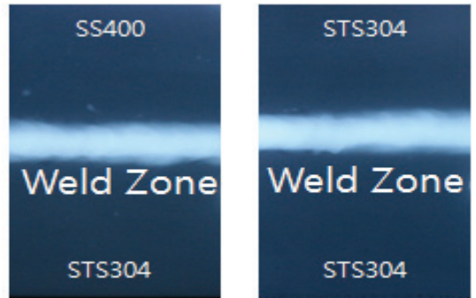
Fig. 5 X-ray topographic of welding defects specimen
