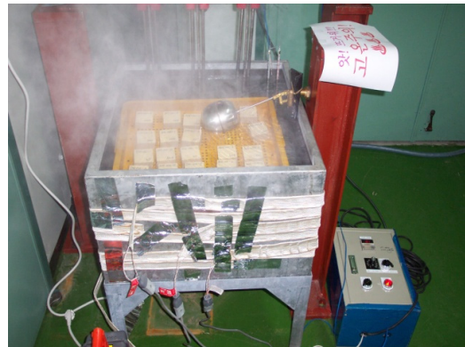
Fig. 5 Accelerated aging apparatus for epoxy coated specimens
