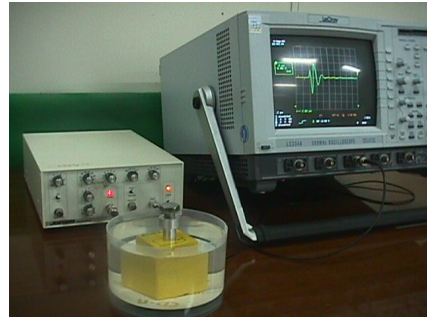
Fig. 6 Experimental configuration for acoustic impedance measurement
