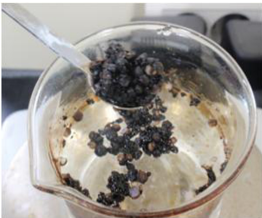
Fig. 7. Oil absorption by composite of silica aerogel and pulps.
