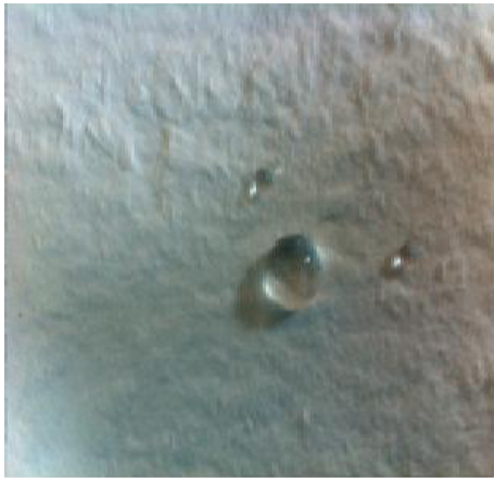
Fig. 5. Hydrophobic effect on the surface of composite of silica aerogel and pulps.
