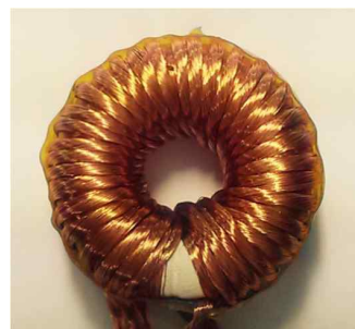
Fig. 10 Experimental toroidal transformer
