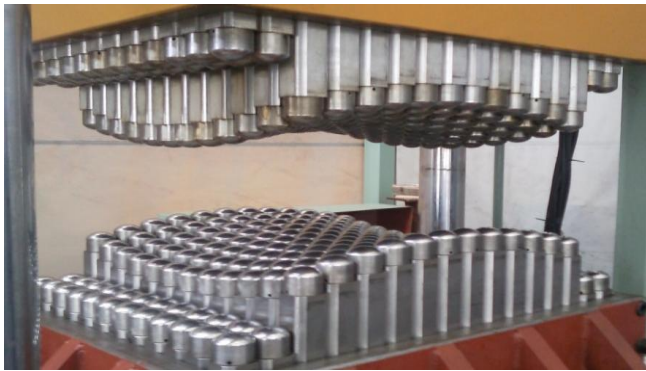
(a) Adjusted flexible die for multi-point forming
