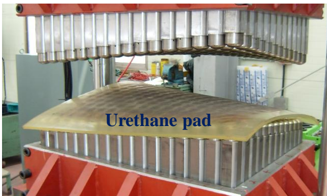
(b) Multi-point forming process using urethane pad Fig. 2 Picture of multi-point forming machine
