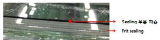
Fig. 8 Detail of Edge Broken
