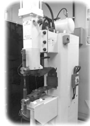
(a) Inverter DC resistance spot welding equipment
