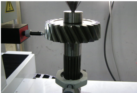
Fig. 7 Profile & lead measurement of the test piece
