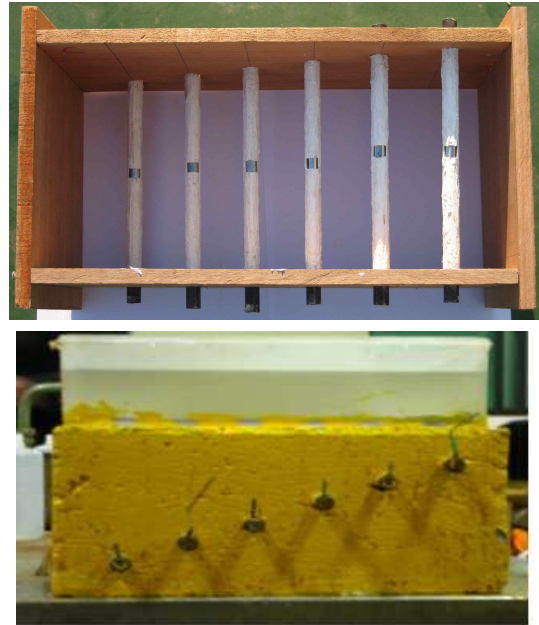
Fig. 1. Mold box for conducting multiple test specimen and completed multiple test specimen for experiment.
