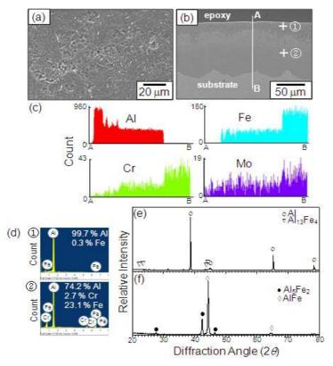
Fig. 2. Al hot dipped T22 steel. (a) SEM top view, (b) cross-sectional SEM image, (c) EDS line profiles of Al, Fe, Cr, and Mo along A-B, (d) EDS spectra of the spot ① and ②, (e) XRD pattern before grinding the surface, (f) XRD pattern after grinding off the outer coating layer.
