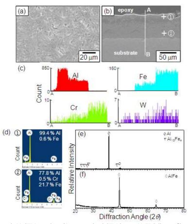
**Fig. 3.** Al hot dipped T23 steel. (a) SEM top view, (b) cross-sectional SEM image, (c) EDS line profiles of Al, Fe, Cr, and W along A-B, (d) EDS spectra of the spot ① and ②, (e) XRD pattern before grinding the surface, (f) XRD pattern after grinding off the outer coating layer.
