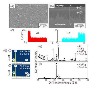
Fig. 1. Al hot dipped low carbon steel. (a) SEM top view, (b) cross-sectional SEM image, (c) EDS line profiles of Al and Fe along A-B, (d) EDS spectra of the spot ① and ②, (e) XRD pattern before grinding the surface, (f) XRD pattern after grinding off the outer coating layer.
