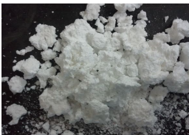
[Fig. 10] Silica power manufactured without the use of surfactants.
