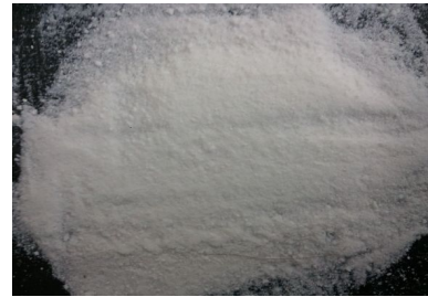
[Fig. 11] Silica powder manufactured with the use of HPC(2.5%)+PEG(2.5%) surfactants.
