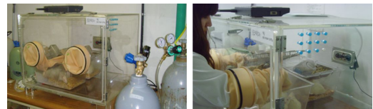
[Fig. 1] Hypoxic and anaerobic comi-incubator. We constructed a hypoxic and anaerobic comi-incubator for establishing in vivo non-lethal hypoxic conditions. We observed the degree of damage by varying the oxygen concentration. This device enabled us to conduct various animal experiments under hypoxic conditions.
