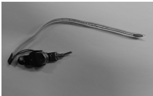
Fig 1. Digital sensor devise for chest compression.
