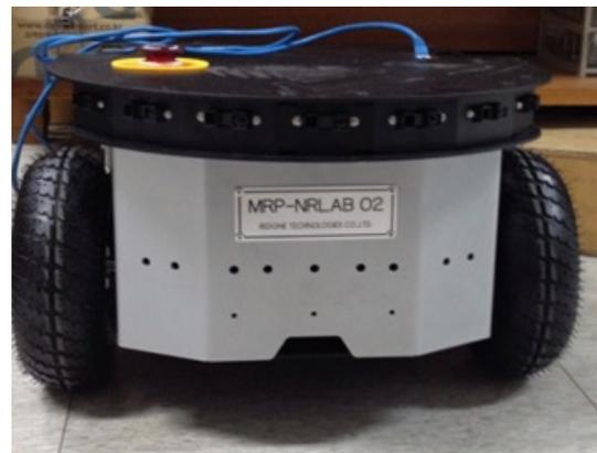
Figure 3. Differential drive robot MRP-NRLAB02.
