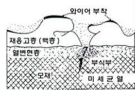
Fig. 7. Wire Electrical Discharge Machining of the damaged layer schematic diagram
