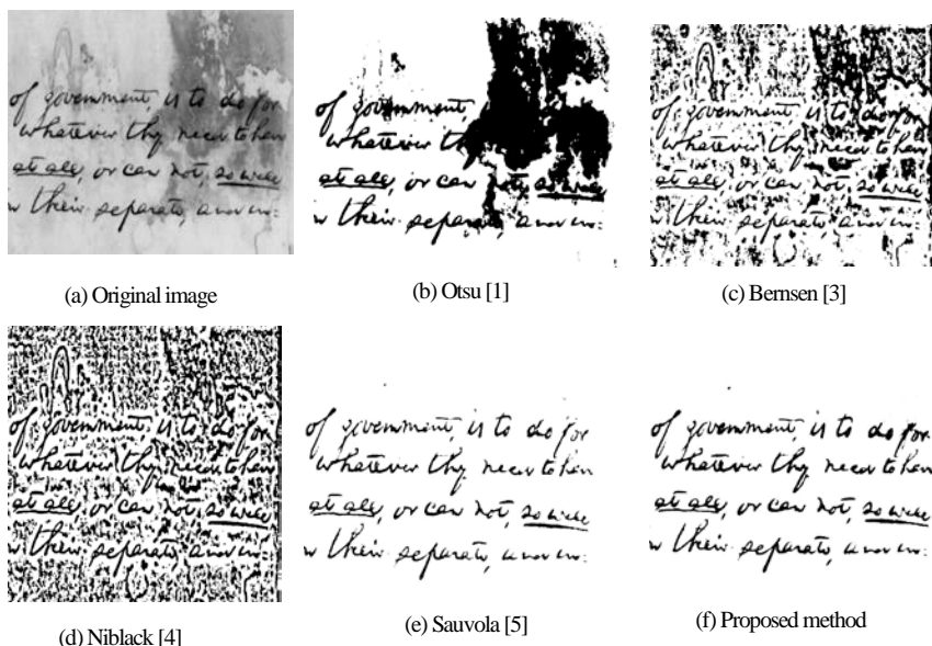
Fig. 10. Comparison of proposed method with other methods: (a) original images, (b) Otsu's results, (c) Bemsen's results, (d) Niblack's results, (e) Sauvola's results, and (f) proposed method's results
