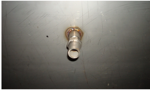
(a) Thermocouple on the ceiling
