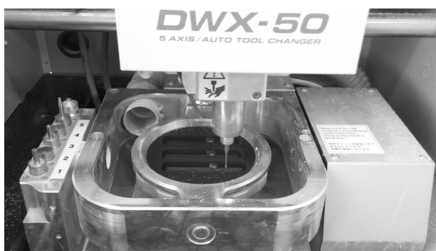
Fig. 4. Milling process of inlay wax blocks for specimens fabricated
