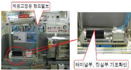
Fig. 5. Leak test of fuel heater
