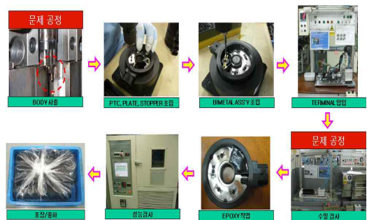
Fig. 9. Block heater assembly and performance evaluation flow
