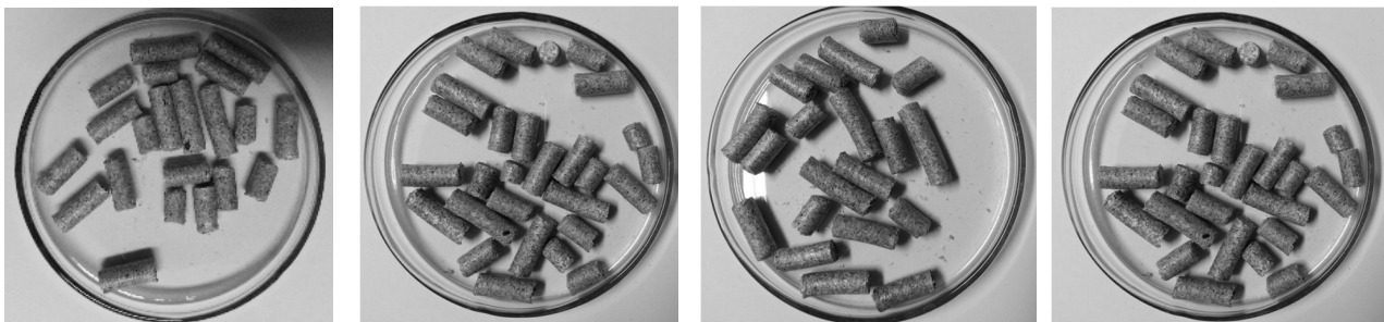
Fig. 4. Images of agropellets fabricated with a) non-treated rape stalk, b) distilled water-, c) acetic acid- and d) oxalic acid-immersed rape stalk.
