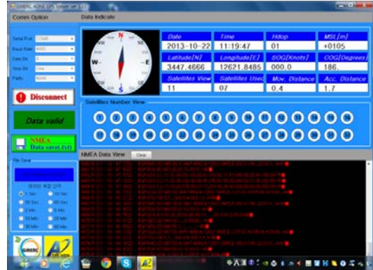
Figure 10: EDiMS software ship speed measurement monitor display
