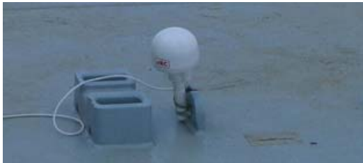
Figure 8: Portable DGPS mounted during speed measurement
