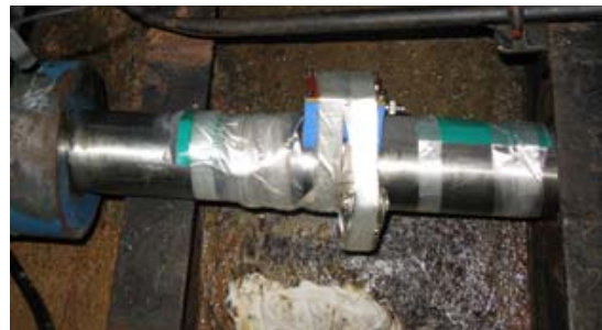
Figure 7: Telemeter system arrangement on 99-mm diameter shaft
