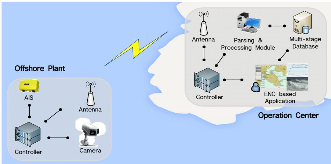
**Figure 2:** Conceptual diagram of offshore remote monitoring system
