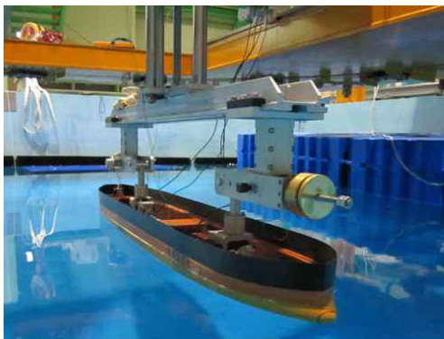
Fig. 4 Model installed on strongback
