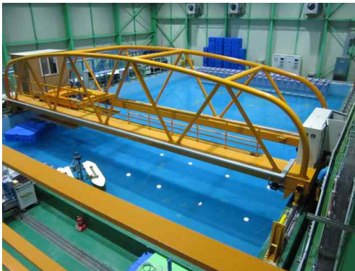
Fig. 1 Square tank and towing carriage in CWNU
