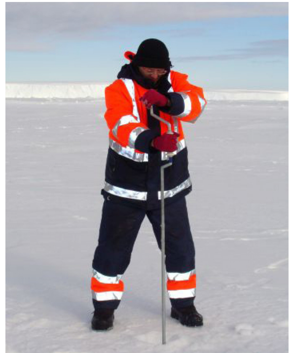
Fig. 1 Sampling of Ice cores by a hand tubular drill
