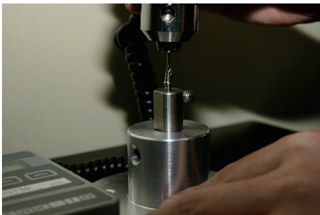
Fig. 2. Detorque values measured by a digital torque gauge.
