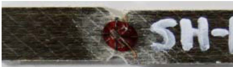
Fig. 6. Specimen after shear test (2-D fabric)
