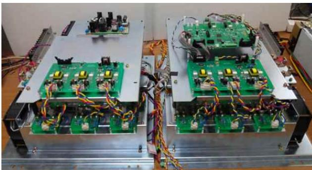
Fig. 11 Prototype of 5kW parallel three-phase bi-directional isolated interleaved dc-dc converter
