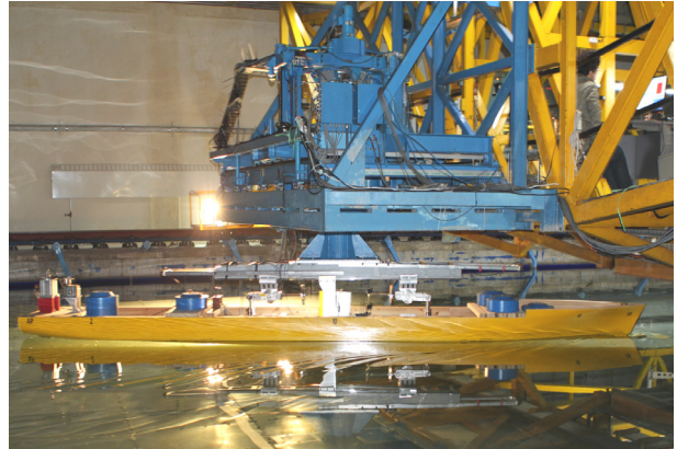
Fig. 6 Captive condition of HPMM device
