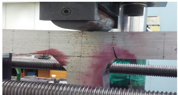
Fig. 4 Toe fracture (fatigue test specimen)
