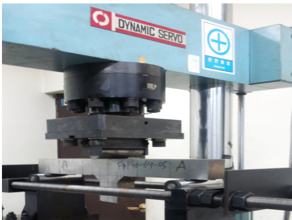
(b) Fatigue test set up
