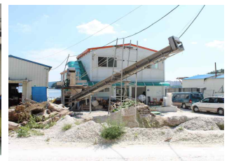
Figure 2. Image of shell crushing equipment
