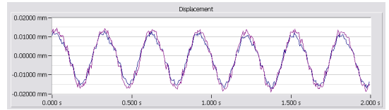
Fig. 13 Vibration displacements of rotating-axis without shape error
