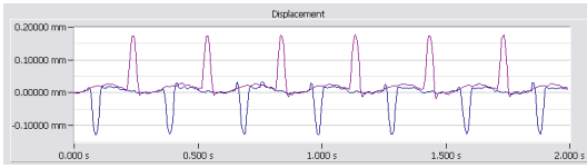
Fig. 15 Vibration displacements of rotating-axis with shape error along one direction
