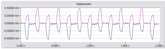
Fig. 17 Vibration displacements of rotating-axis with shape error along two directions
